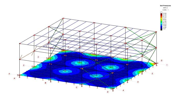
The analysis of the model allows to calculate several important parameters for the design of the foundation. While considering the various load combinations, the nodal displacements of the slab on the ground make it possible to check the stability and deflections of the structure.
