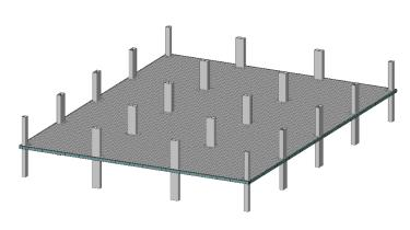
The deflections of concrete slabs are composed of: immediate deflections and time-dependent deflections. The immediate deflections are calculated for the selected load combinations. The shrinkage and creep phenomenon are time-dependent effects causing deflections over long periods of time. The overall deflections of the building is a combination of both the immediate and time-dependent deflections.
