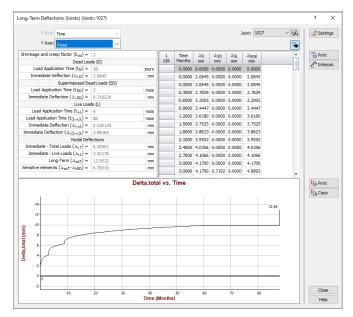
In order to calculate the service limit state, SAFI GSE automated the slab spans detection. For each load combination and span, the Serviceability Limit State (SLS) ratio is calculated using the long-term deflections and the span length and compared to the relative deflection limits (L/x) defined by the user. The user may easily verify if the serviceability limit states are respected or if more reinforcements are required in some portions of the slab.
