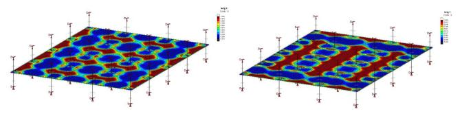
The time-dependent deflections are calculated using the cracked concrete immediate deflections of the specified load combinations. In SAFI, the load combinations management for the cracked concrete deflections has been automated. The CSA A23.3 proposes the following equation to calculate the long-term deflections. The ACI 318 equation is very similar.
