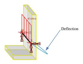
Also, the deflection criteria and the limit states calculation for the deflections with an alpha  $(\alpha)$  angle different than zero are now done on the straight axes.
