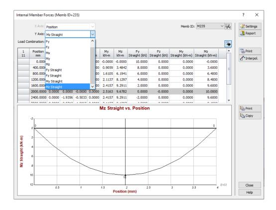
The forces and moments on the straight axes can also be visualized on the structure in the main window. For example, for a simply supported single angle with vertical loads, the moments on the strong and weak axes are both different than zero, as displayed below. Note that the steel design for bending moments are always done according to the principal axes.
