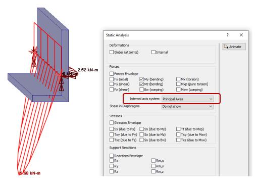
For the same example, the bending moments according to the straight axes is only around the Mz axis and the My value is zero, as displayed below.
