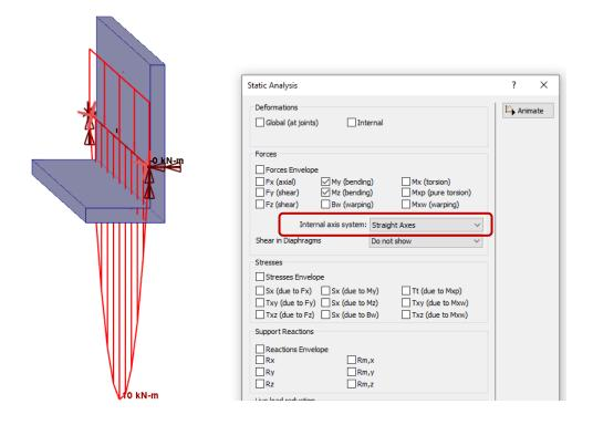
Note that the design for the shear limit states for steel is always done according to the straight axes. So, the associated forces are Fy and Fz on the straight axes.
